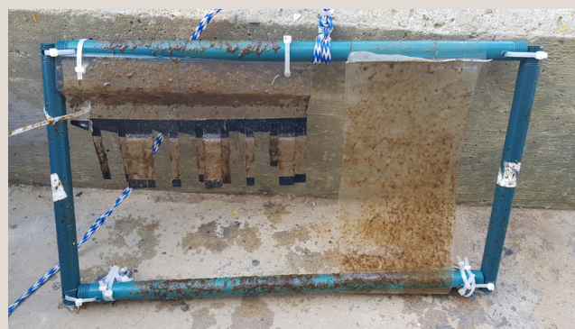
Figure 2: Polycarbonate (left) and plastic (right) sheets after diatom settlement (T14).
