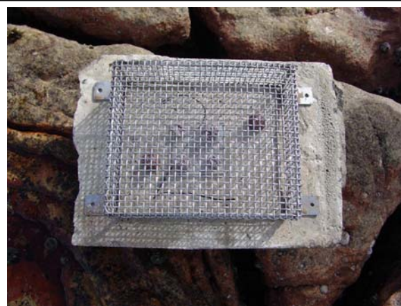
Figure 3. Stainless steel cages were mounted onto concrete slabs wherein the experiment was housed. Control winkles were caged in along with the mounted treatments.
