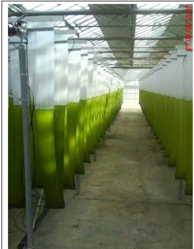
A photobioreactor power plant operated by RWE, Germany's second-biggest electricity company (image source: http://www.engineeringnews.co.za/ ).
