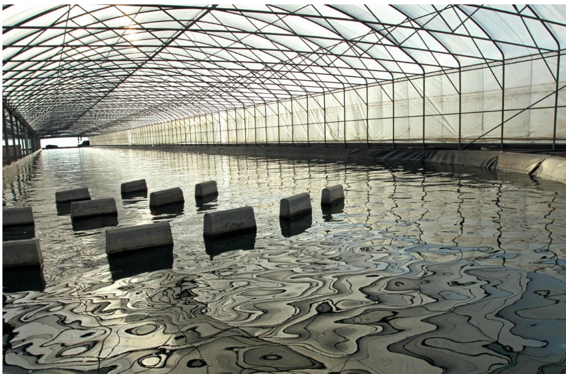
CeBER pilot large scale (500 000 L) Spirulina cultivation at the BioDelta site in Franschoek (Photo: Candice Mazzolini)
